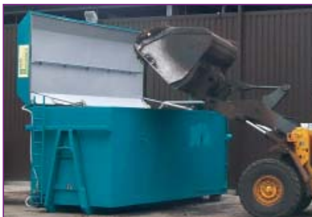
Sirocco in-vessel composting unit – 2.5 × 2.5 × 5 metres
