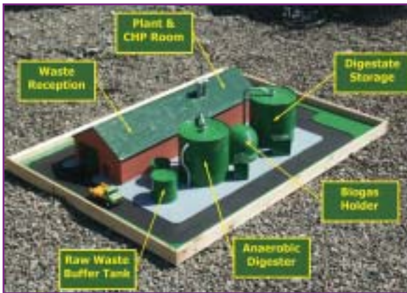
Model of 2,500 tpa Anaerobic digestion plant for food waste
