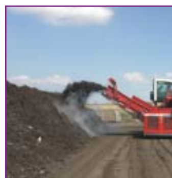
Side turner, Pitsea composting site
