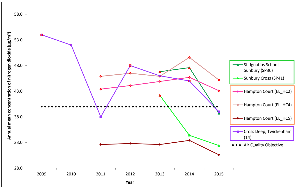
Figure 7-3: Annual mean concentration of NO 2 (µg/m 3 ) from monitoring stations within SBC (green box), EBC (orange box), and RBRUT (purple box) AQMAs. (Codes in brackets correspond with the respective borough's air quality report and are marked on the baseline maps; data points outlined in red signify a concentration above the AQO).
